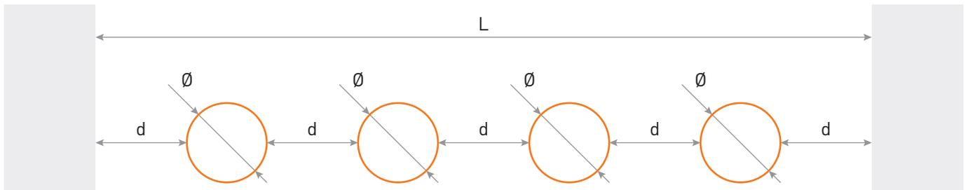
$$N = \frac{L - d_{\text{recommended}}}{\varnothing + d_{\text{recommended}}}$$
